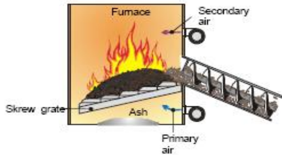
SCREW GRATE WITH HORIZONTAL FEED
